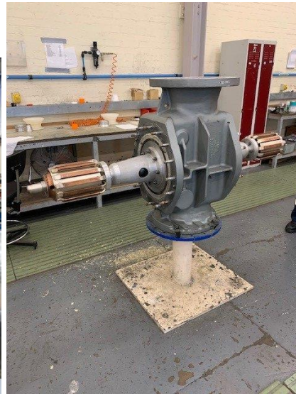
Figure 7.4: 400kV AIS Gas Circuit Breaker Refurbishment with new sealant applied
