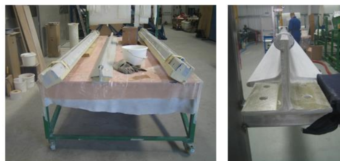
Mould split leaving final part with bare ends for attachment plates
