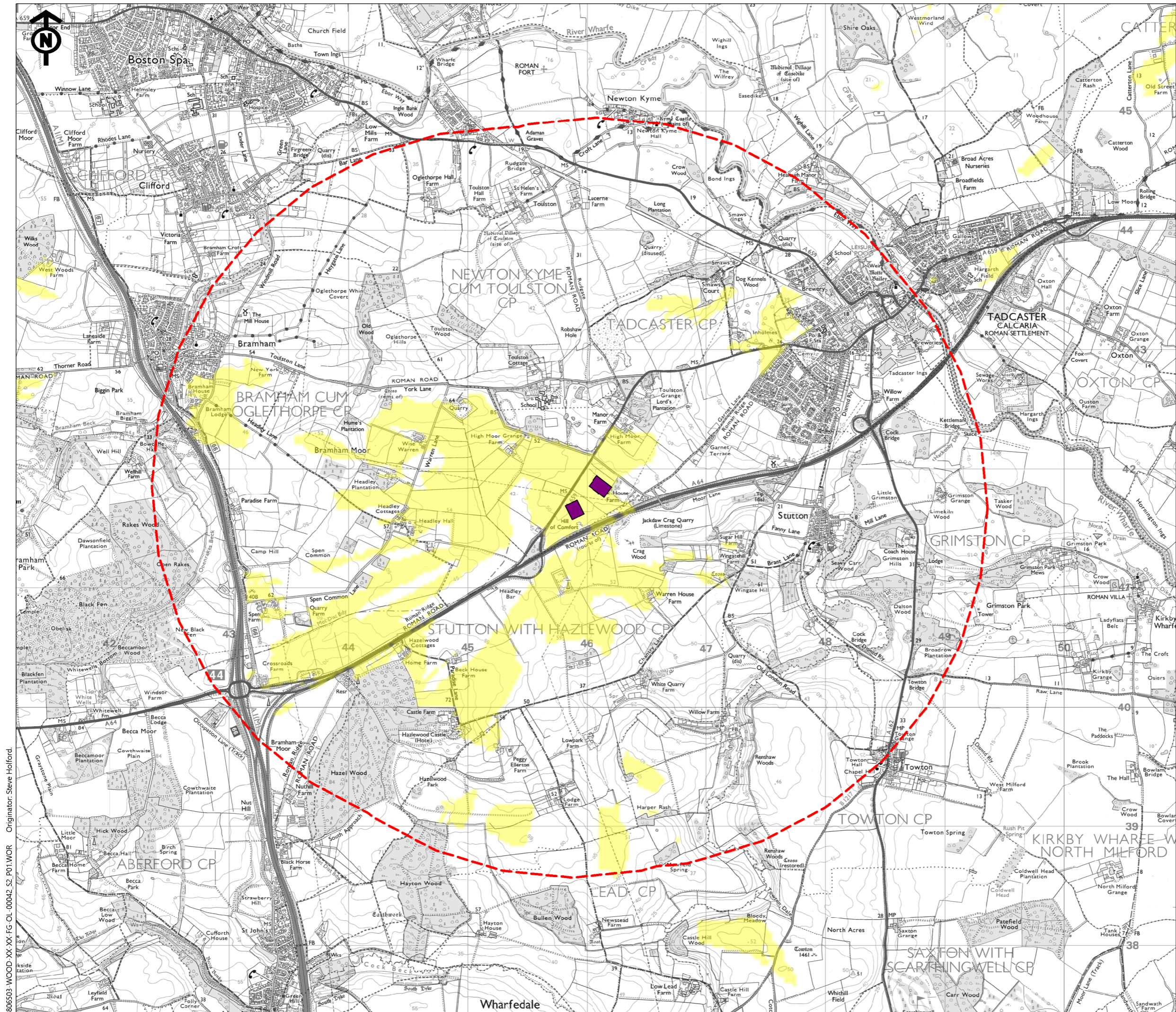
Figure 6.8 Zone of Theoretical Visibility of Tadcaster Temporary Construction Compounds
