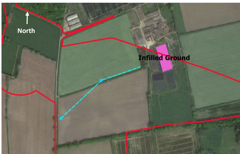
Figure 10A.4: Sewer and infilled ground at land parcel 1230
