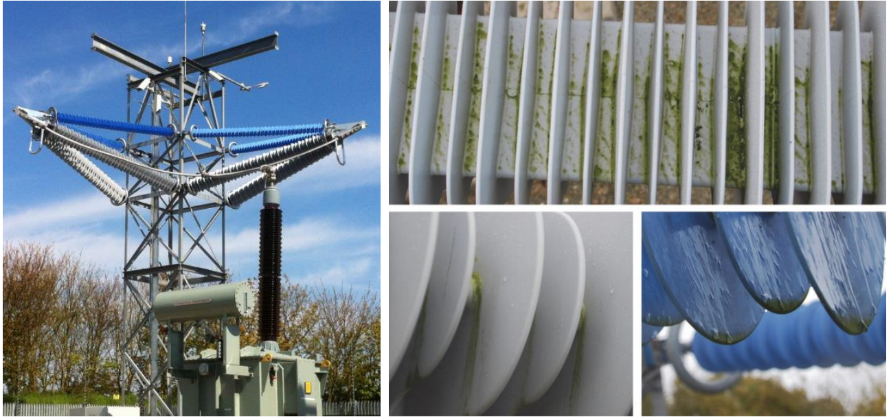
Figure 6.4 - Live trial site (left) [74] and algae growth on the ICA insulators 35 months (right) [75]
