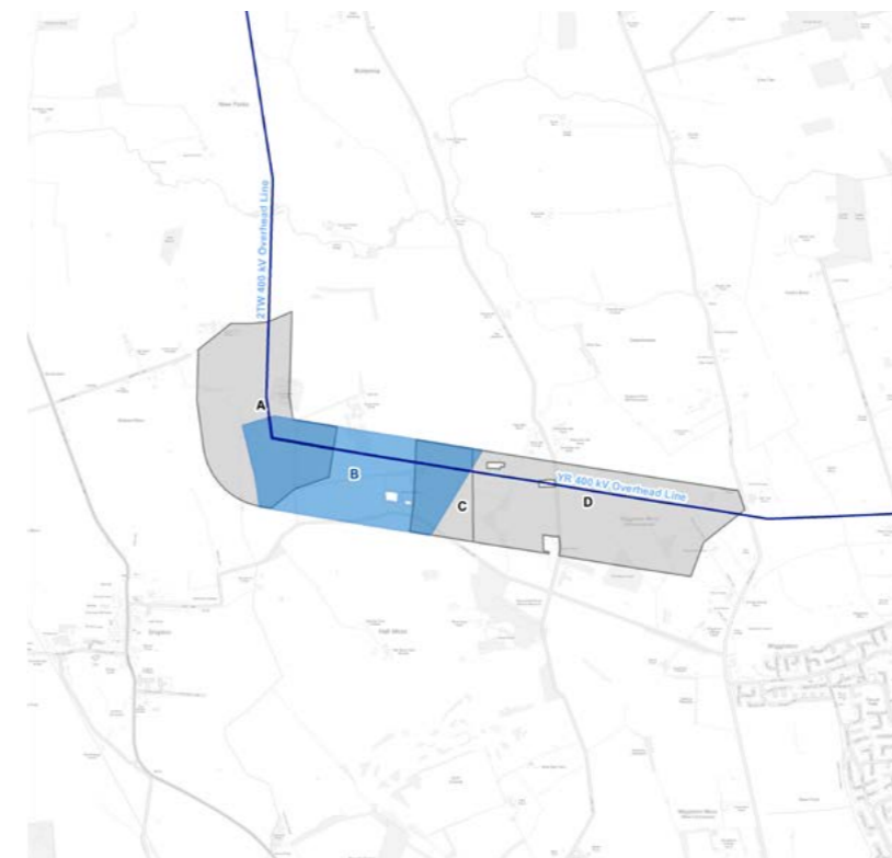
Figure 5 – Siting areas considered for two proposed cable sealing end compounds and associated infrastructure
