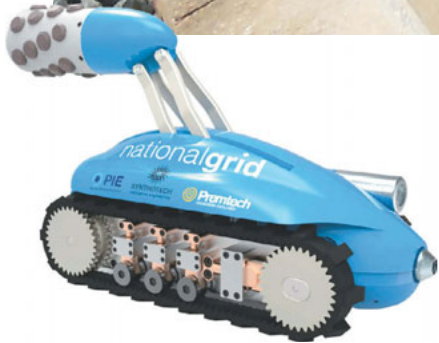
The 15 by 10-inch robot has a dolphin-nose design to reduce drag and friction
