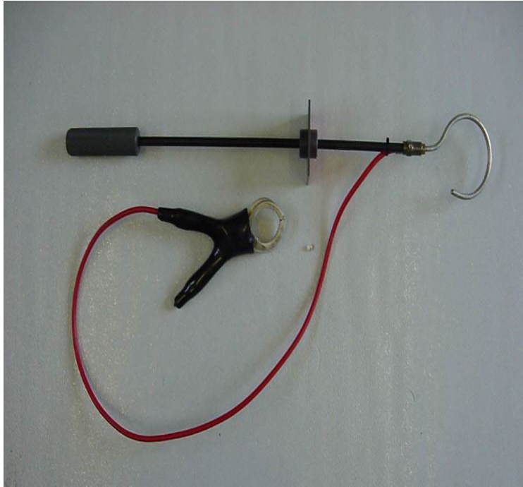
Figure 5.2D – Discharge Stick with single 'crook' end.
