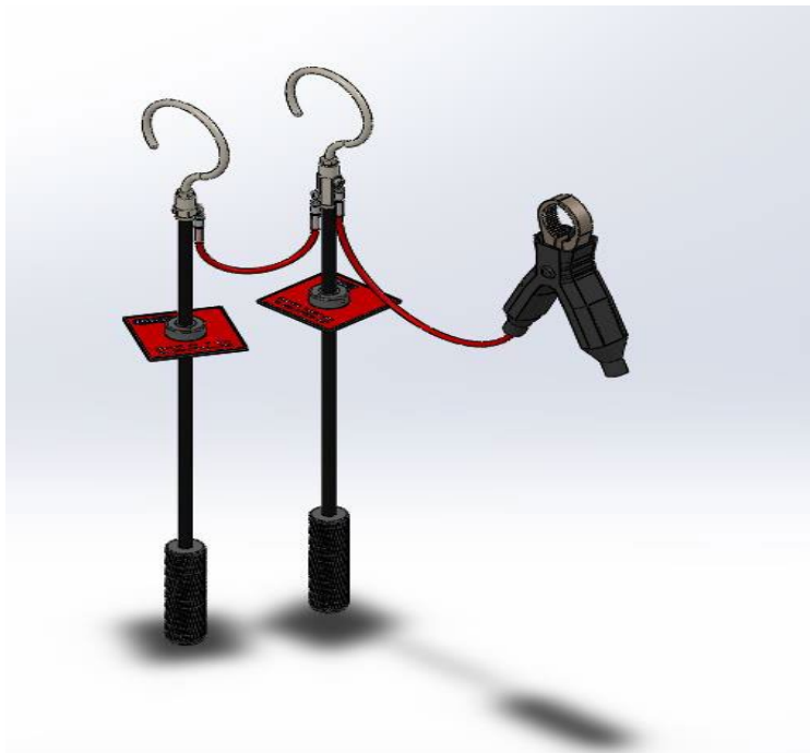
Figure 5.2E – Discharge Stick with dual 'crook' ends.
