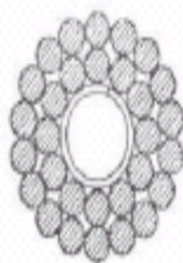
Figure 4.1A - Holtom Type Copper Conductor
