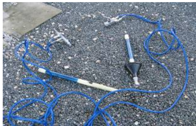
Figure 6.1A - Temporary Earth Bond and Temporary Earth Bond Pole
