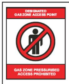
DESIGNATED GAS ZONE ACCESS POINT NOTICE (DISPLAYING GAS ZONE PRESSURISED ACCESS PROHIBITED)
