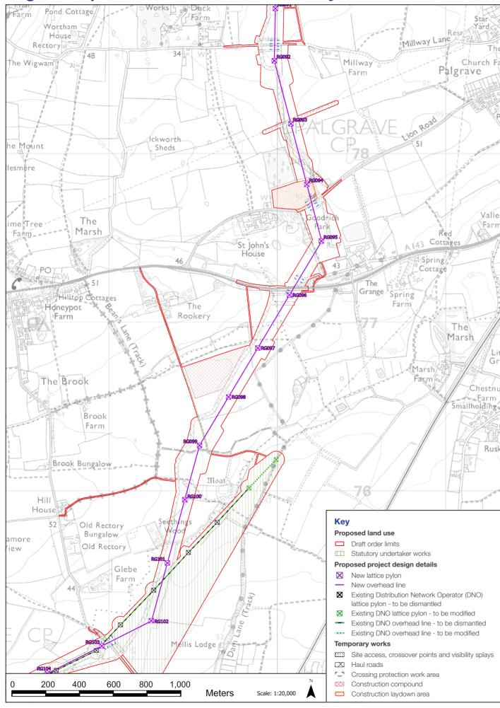
To accommodate this proposed change in alignment, we are also proposing to move the haul road and the bellmouths - where project traffic would cross public highways or enter the project site. We're now proposing to reposition the bellmouth that would cross the A143 Old Bury Road to the east of its previously proposed location.
