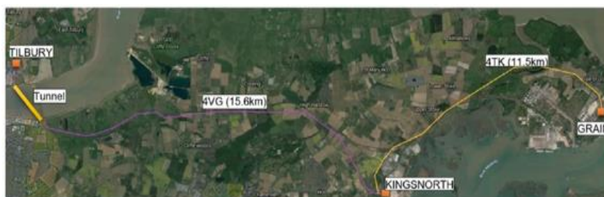
Figure 1: This is the aerial view of the intended connection from Tilbury to Grain. The coloured lines represent the circuits between each substation. Tilbury – Kingsnorth (purple) and Kingsnorth to Grain (yellow). The tunnel is represented with a thick yellow line.
