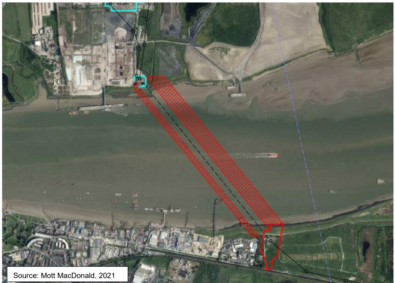
Plate 2-3: Option 2, existing Tunnel (black dashed line) and two indicative corridors for new tunnel (red hatched areas).
