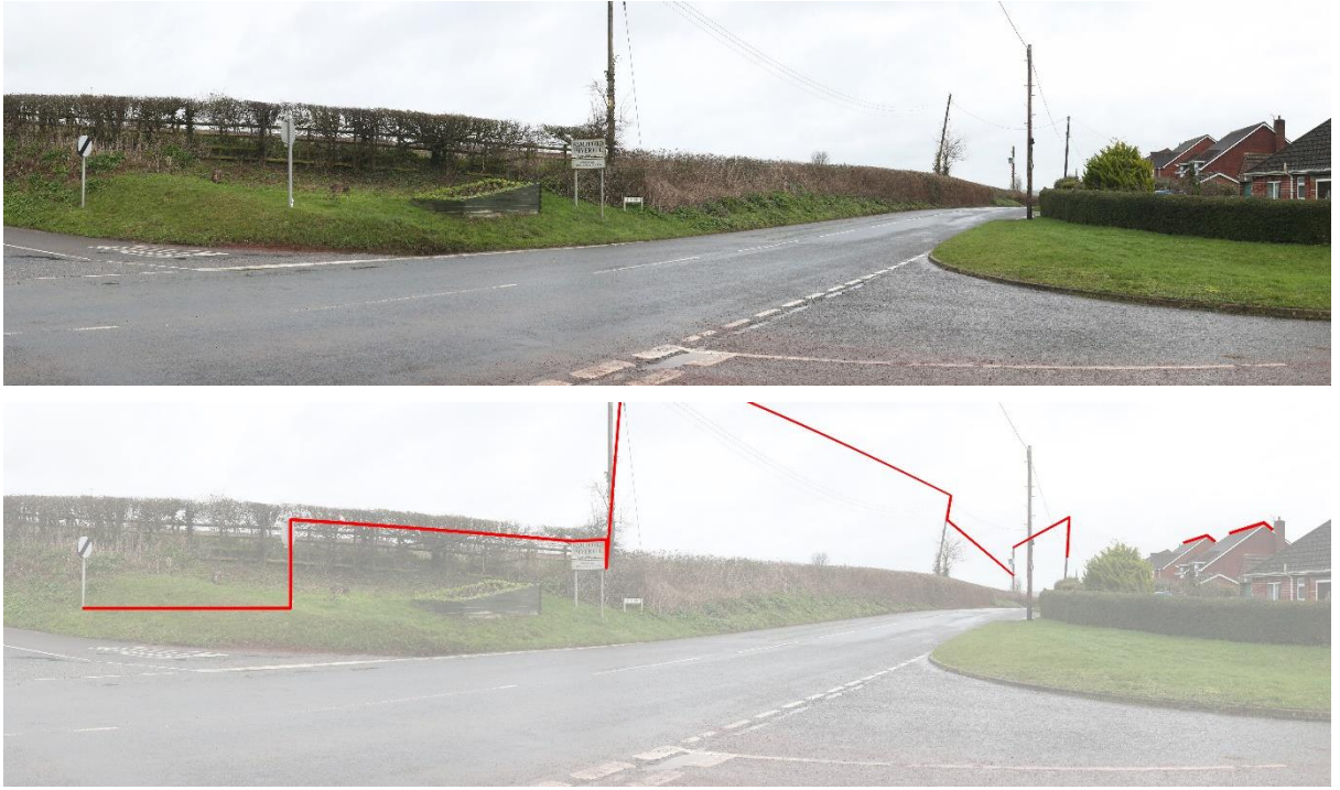
Image 3.2.A. 1 Photographs illustrating an existing photograph (top) and typical reference line connecting surveyed points (bottom)
