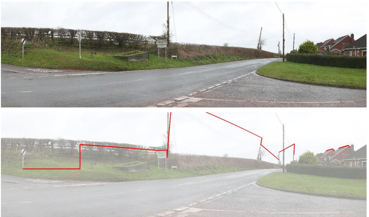
Image 2.2.A.1 Photographs illustrating an existing photograph (top) and typical reference line connecting surveyed points (bottom)
