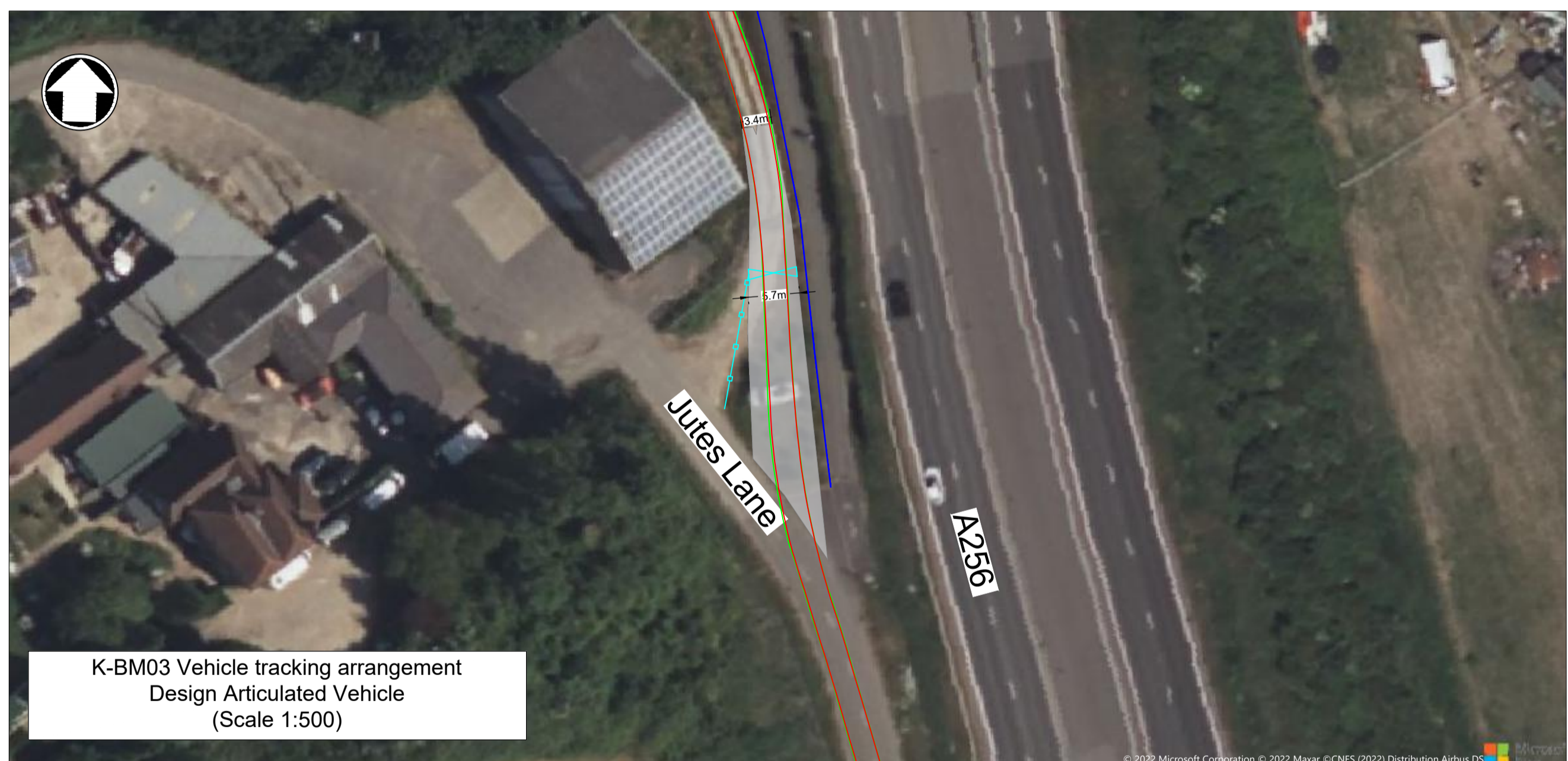
K-BM03 Vehicle tracking arrangement Dennis Sabre Fire Tender (Scale 1:500)
