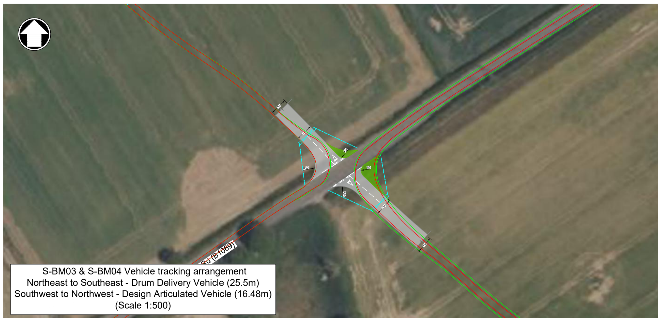
S-BM03 & S-BM04 Vehicle tracking arrangement Northeast to Northwest - Drum Delivery Vehicle (25.5m) Southwest to Southeast - Design Articulated Vehicle (16.48m) (Scale 1:500)
