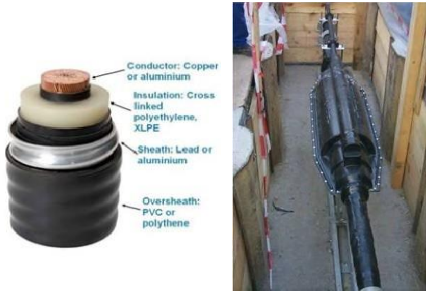
Figure C.4: Cable Cross-Section and Joint
