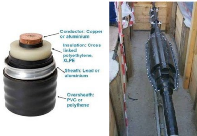
Figure C.4: Cable Cross-Section and Joint
