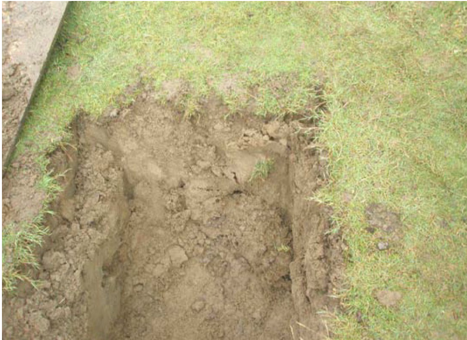
Plate 15.4: Trial pit at edge of saltmarsh, TP04 (Norwest Holst, 2009)
