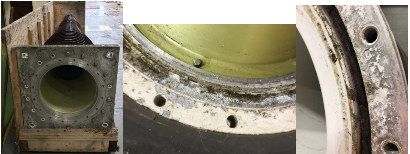
Figure 10 – Photos of leaking T155/1 bushing
