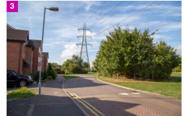
3 The use of planting and the meandering road alignment changing viewing angles help to reduce the visual prominence of the pylon. A raised table and change in materials add a degree of sensory richness while also assisting with traffic calming.
