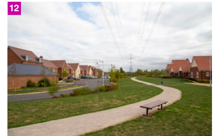
12 The meandering pathway changes people's line of sight when moving through the space, reducing the perceived linearity of the transmission line. Planting and the design of the adjacent housing provide sensory richness and distract positively from the visual prominence of the pylons and overhead lines.
