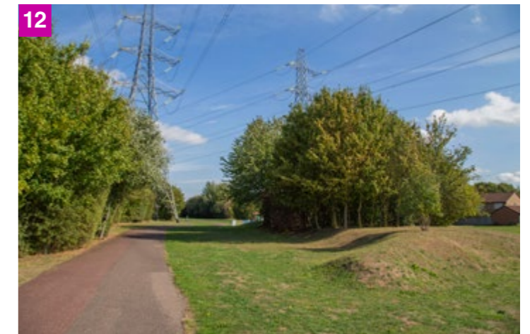
12 Localised sculpting of landform elevate belts of planting to subtly increase their screening effectiveness. Planting has been arranged to wrap around the bases of pylons to limit visual exposure while maintaining free access for maintenance. Formal play space is integrated beneath the overhead lines.
