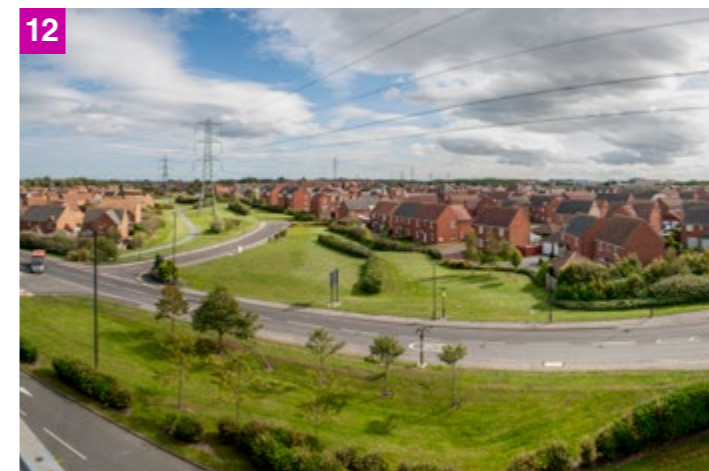
The linearity of transmission line is reduced through the use of a number of design mechanisms including the effective use of informal planting beds, meandering path and road alignments and the staggered arrangement of building frontages and rooflines.
