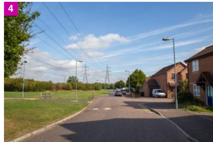
4 The foot and cycle way connections have been designed to coincide with the street layout of the housing development. A raised table provides level, pedestrian-prioritised access. A mature vegetation belt works well to screen views of the base of the pylons.
