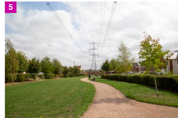
5 The open space beneath the overhead lines provides opportunities for informal recreation with shrub and tree planting providing visual interest, biodiversity value and a degree of visual distraction to reduce the impact of the pylons.
