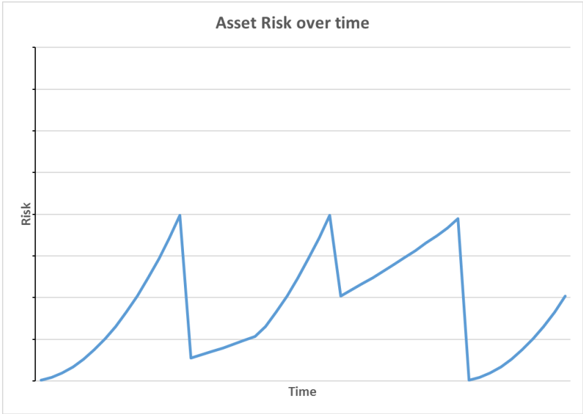
Figure 8. How asset risk changes over time and is affected by maintenance activities and ultimately replacement
