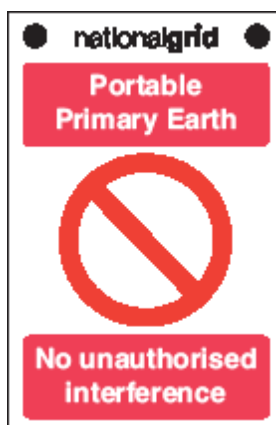
Figure 4.7 – Example of Portable Primary Earth Label
