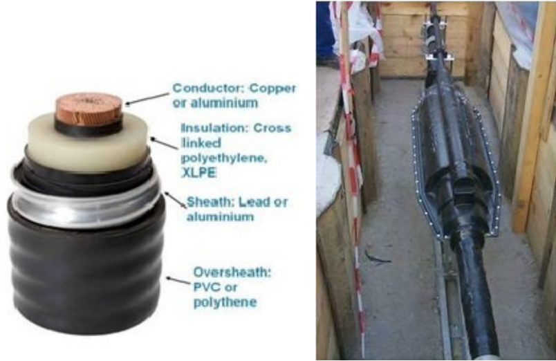
Figure C.4 – Cable Cross-Section and Joint
