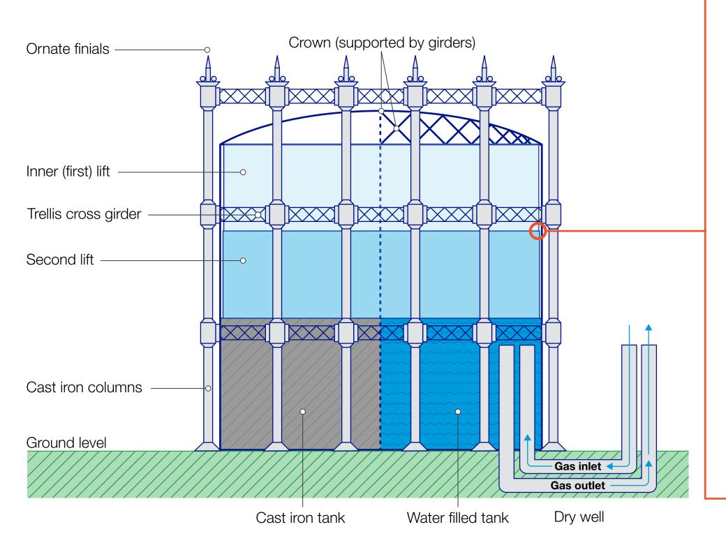
The cup and grip mechanism shown, provided a watertight seal between each lift, keeping the gas within the gasholder as the lifts engaged. Cups and grips could be rounded (as shown) or rectangular.
