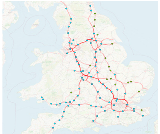
HGV traffic density overlaid with MSAs ( blue ) and selected TRSAs ( green ) for en-route HGV energy provision.
