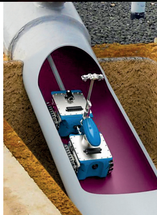
Pictures shown above GRAID robot developed for use in high-pressure underground gas pipelines.
