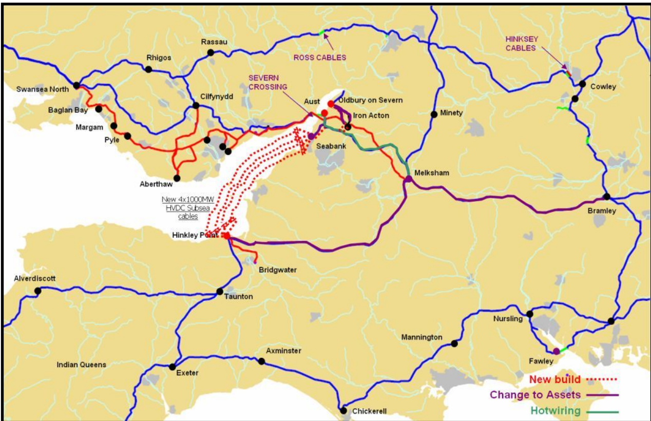
3.21 Option H6 and H20 were options connecting Hinkley Point with Aberthaw in South Wales via AC and DC subsea cables, over a distance of approximately 60km.
